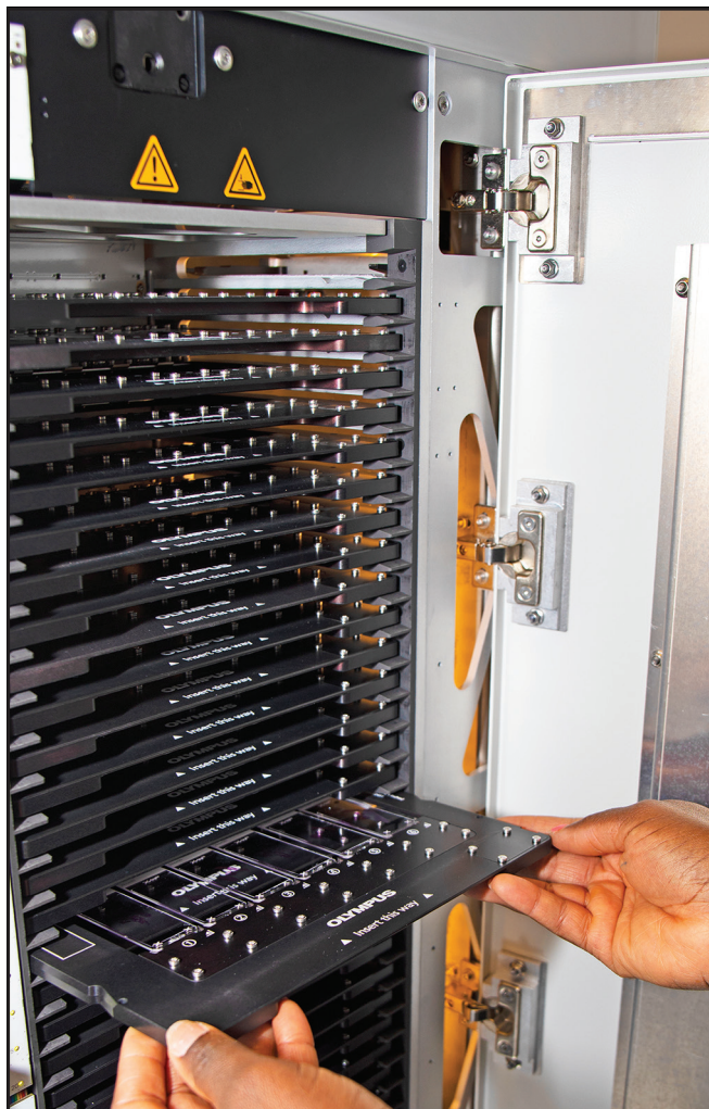
Figure 2. Internal view of digital slide scanner showing racks of slides and capacity. Courtesy of LTC Christopher Schellhase.
